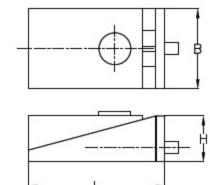
The Smooth Sliding Block is a device for fine and stepless height adjustment.
