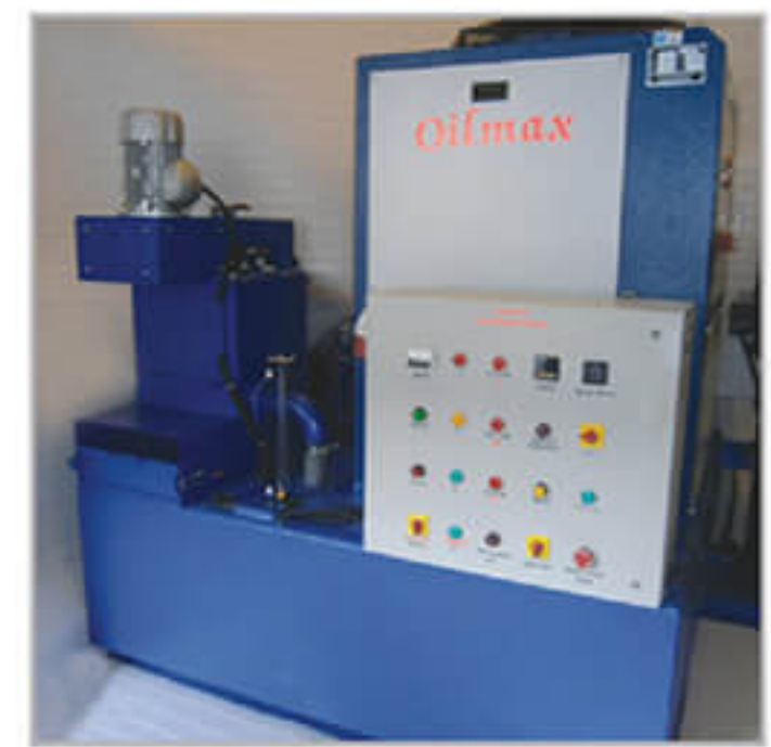
Centrifugal Oil Cleaner (with Chiller)
